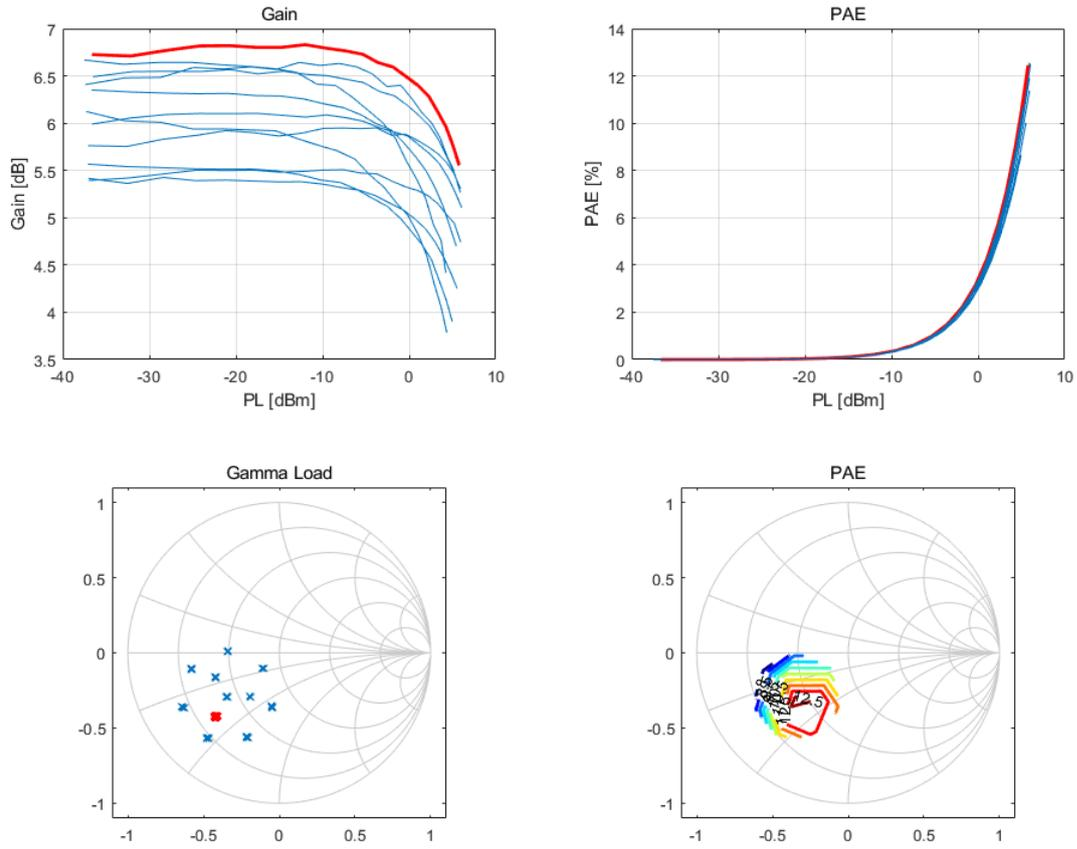
Figure 4. Load pull results at 140 GHz when the HEMT was biased with  $V_g = 0.1$  V and  $V_d = 0.9$  V.
