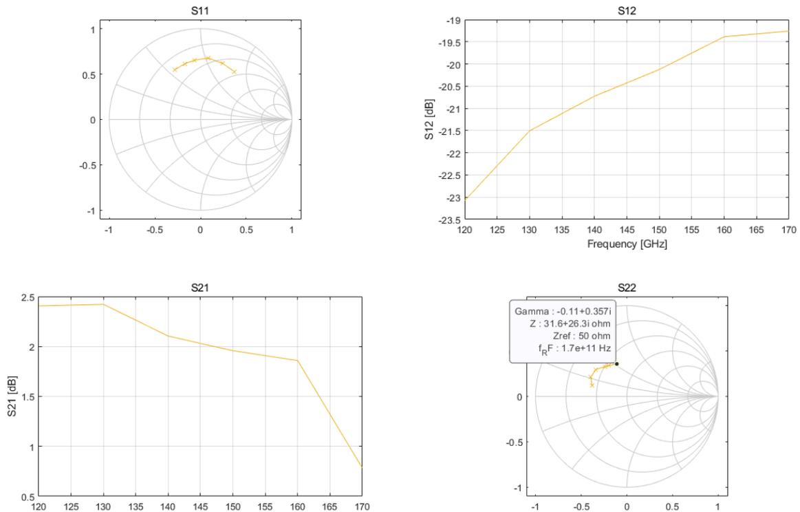
Figure 3. S-parameter of the commercial HEMT when it is biased at with  $V_g = 0.1$  V and  $V_d = 0.9$  V.
