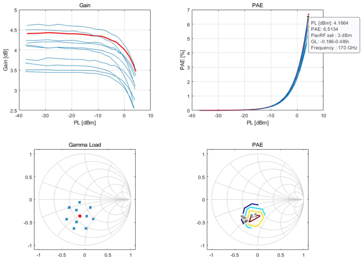
Figure 5. Load pull results at 170 GHz when the HEMT was biased with  $V_g = 0.1$  V and  $V_d = 0.9$  V.
