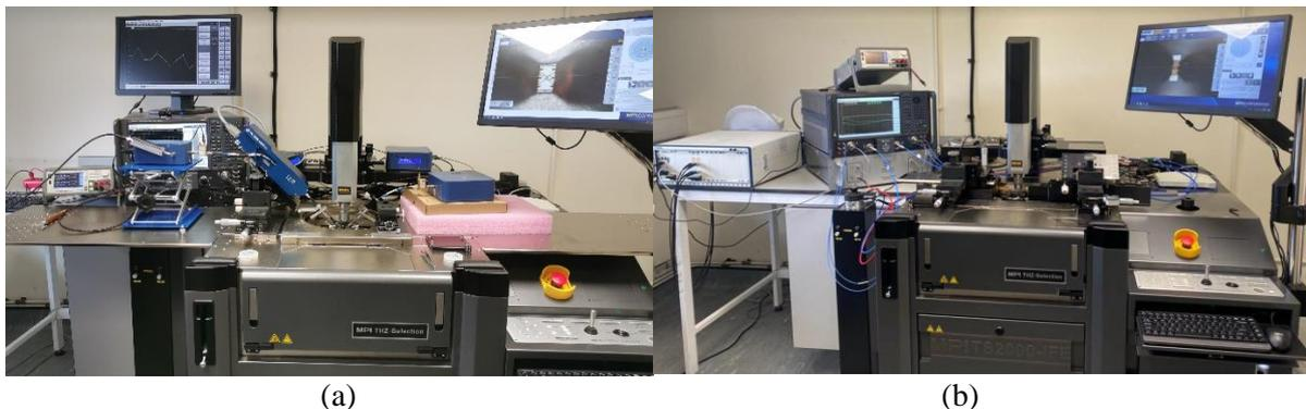
Figure 1. Images of part of the TiC6G on-wafer test cluster for (a) noise parameter measurements between 2 GHz and 50 GHz (b) active load pull test system operating between 110 GHz and 170 GHz.
