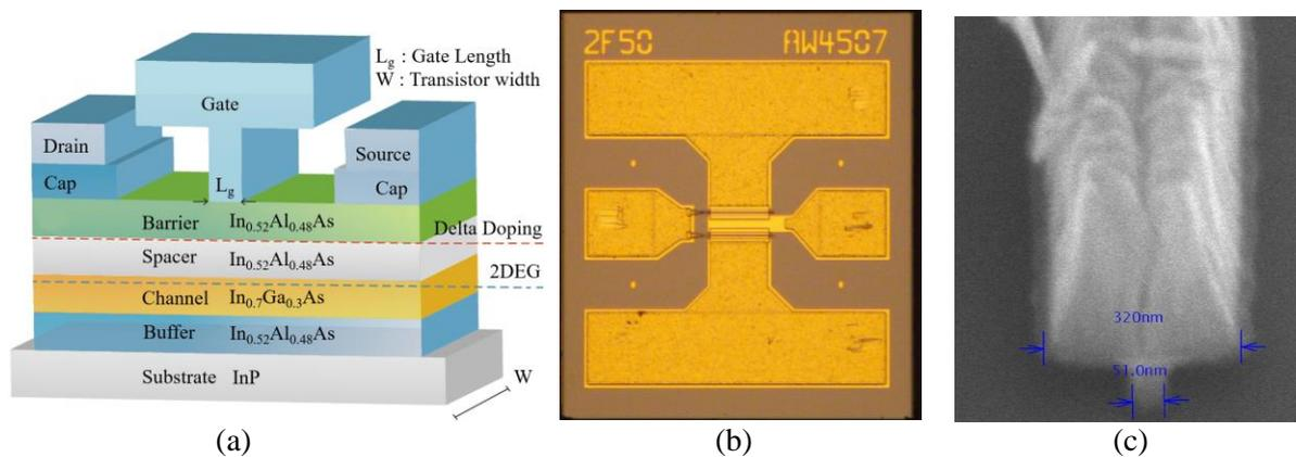
Figure 2. (a) Illustration of the epilayers of a typical pHEMT [1], (b) micrograph of the commercial HEMT die that has 2 fingers and a total of 100  $\mu\text{m}$  width, and (c) Scanning electron microscope (SEM) image of a 50 nm T-gate fabricated at the University of Glasgow [2].
