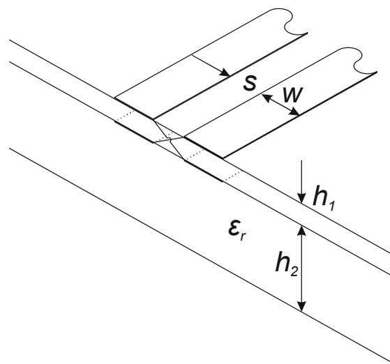
**Fig. 1** Diagram of the Overlay Microstrip Coupler
