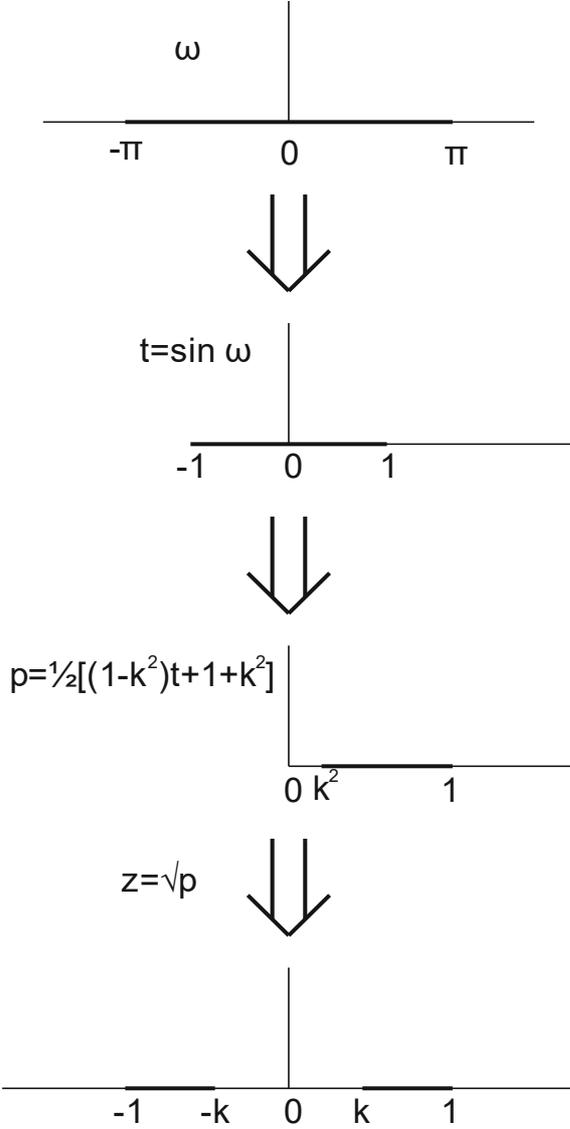
**Fig. 9** Transformation to Even Mode Strips
