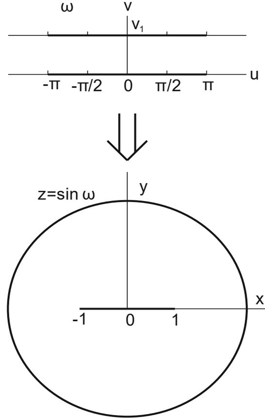
**Fig. 7** Transformation from Parallel Plate to Elliptic Coax
