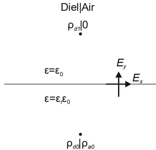
**Fig. 4** Line Charge Parallel to Dielectric Boundary
