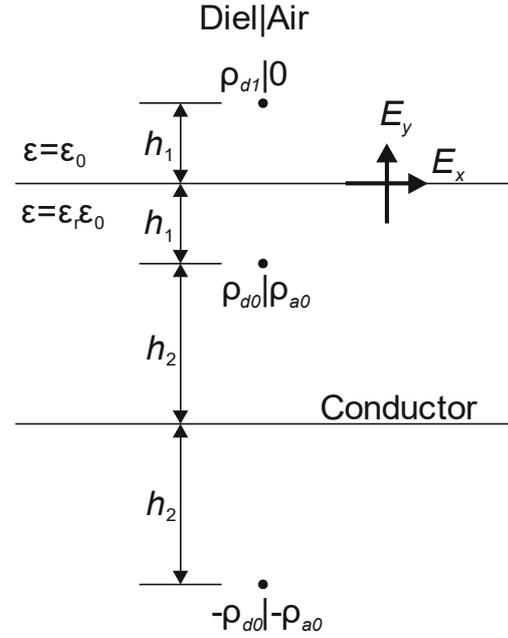
**Fig. 5** Initial Images Created by Dielectric Boundary and Conductor Plane
