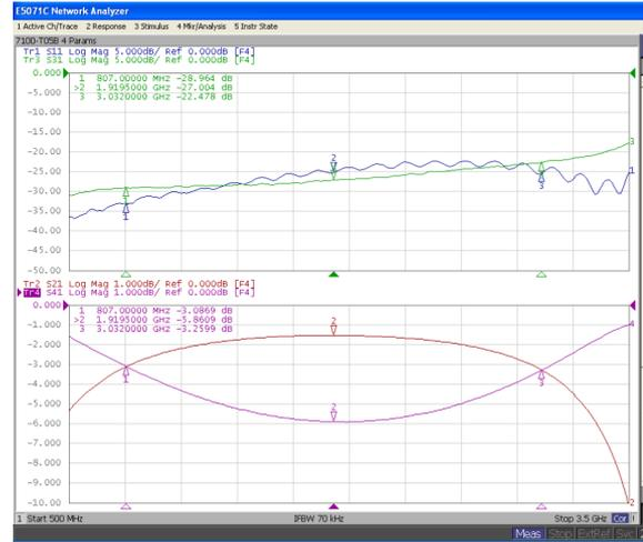
**Fig. 13** Measured Performance of a Practical Coupler
