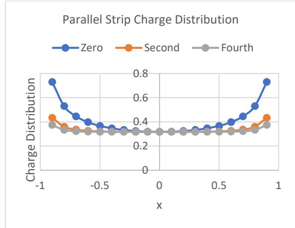
**Fig. 8** Charge Distribution with Increasing Approximation Order
