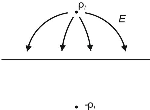
**Fig. 3** Electric Field due to a Line Charge over Conductor
