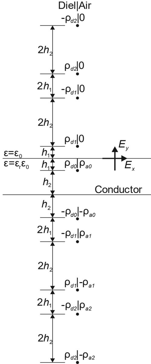
**Fig. 6** Images Propagated by Line Charge in Dielectric
