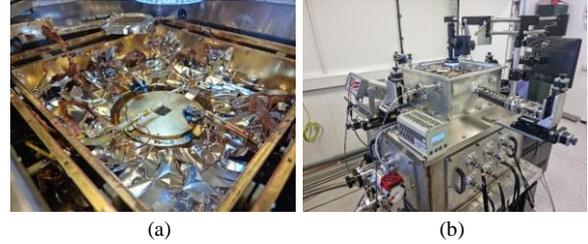
**Figure 7:** Measurement set-up showing the cryogenic probe station: (a) internal view showing the probe arms and the DUT chuck; and (b) external view.
