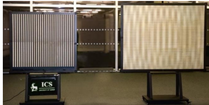
Fig.2 The world’s first RIS demo at 6GIC. The left-side one can dynamically change the beam while the one on right has fixed reflected beam with no need of electrical power.
