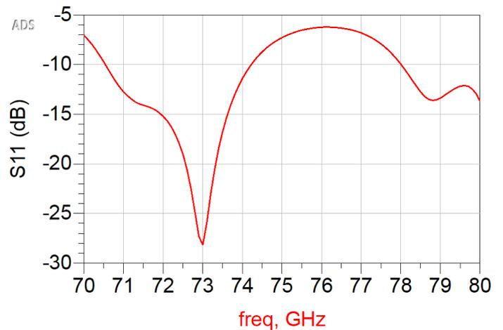
Fig.5. Measured  $S_{11}$  (dB) of the Antenna Array.
