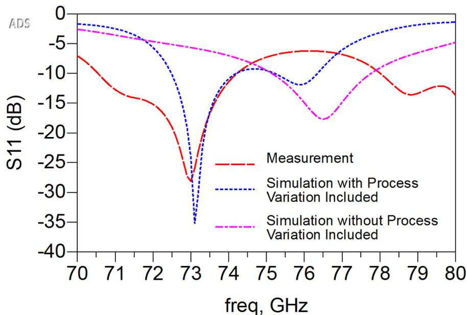
Fig. 8. Change in simulated  $S_{11}$  resonant frequency of the antenna array due to process variation which is verified with the measurement.
