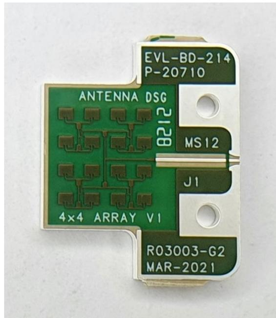
Fig. 2. Fabricated prototype of the proposed microstrip patch antenna array.
