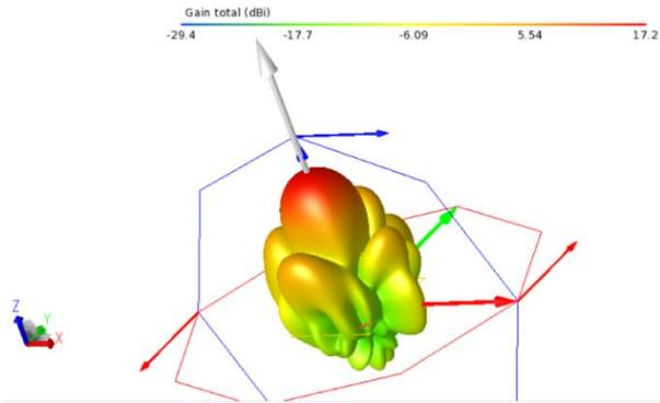
Fig.6. Simulated Radiation Pattern at 76.5 GHz
