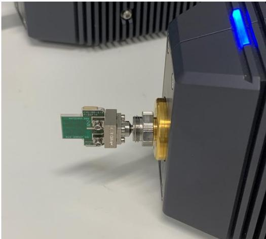
Fig.4. Measurement Set-up of the Antenna Board
