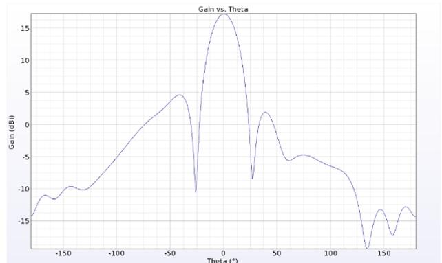
Fig. 7. Simulated Peak Gain in Broadside (dBi) at 76.5 GHz
