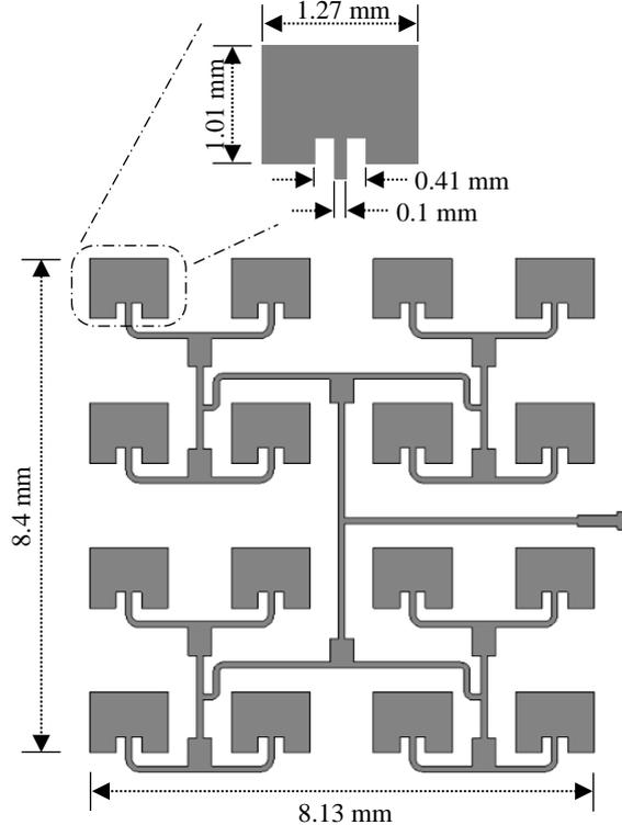
Fig. 1. Design geometry of the proposed 4×4 microstrip patch antenna array.
