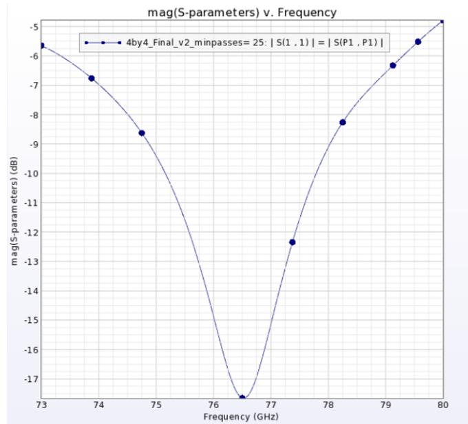
Fig. 3. Simulated Input Return Loss (dB) of the Antenna Array.
